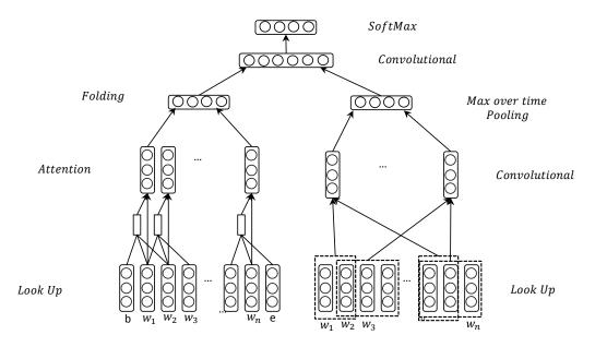
Figure 1: The architecture of the attention-based Convolutional Neural Network
