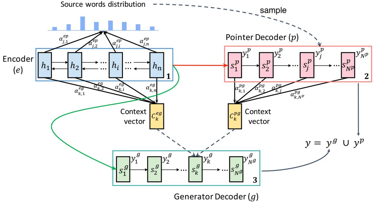
Figure 2: Overall architecture of our novel encoder-decoder model. The pointer decoder ( $p$ ) first extracts words directly from the source text via copying mechanism. Then, the generator decoder ( $g$ ) generates words from a fixed-size output vocabulary. Finally, we combine the outputs of the two decoders as the final result. For simplicity, we omit some links for computing the attention score  $\alpha$  (see sections 3.3 and 3.4 for more details).
